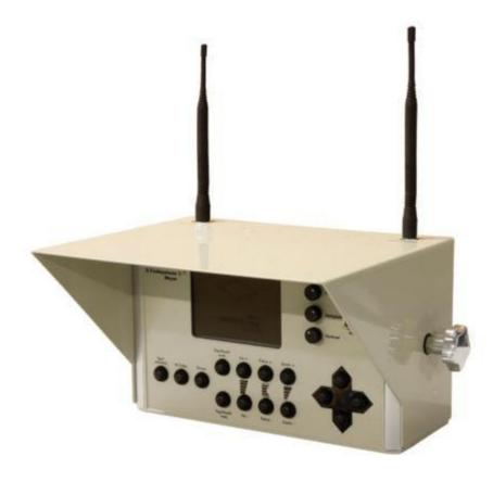
In connection with the operations station. Vehicle 12 V = 11 - 30 V vehicle connection
