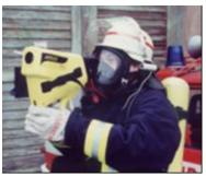
The mobile unit helmet camera combined with an infrared camera and separate bidirectional speech connection for application management is particularly suited for applications in buildings, cellars and tunnel areas as well as for rescue applications in the open terrain.
